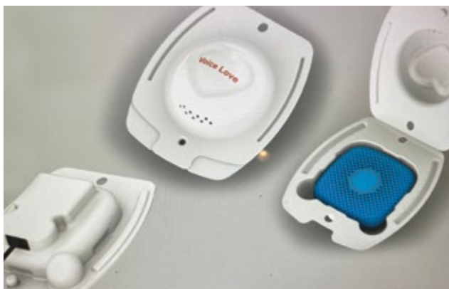
To make Relay’s off-the-shelf consumer device appropriate for medical settings, Schiffman and Fenster had a plastic case designed to protect the small speaker from cross-contamination.
