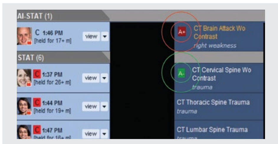
The AI and workflow vendors created a red (positive) and green (negative) badging system that clearly displays the algorithms findings. In this example, the algorithm detected right weakness but not trauma.
