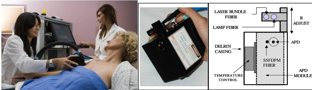
Figure 1 –DOSI instrument (left), with a blowup of the handheld probe (middle). The DOSI instrument is a handheld, single spatial point spectroscopic imager that combines discrete frequency-domain and broadband steady-state spectrometers, with a schematic of the device (right).
