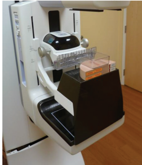
Figure 27. Position of attenuator for Automatic Exposure Control System Performance test in magnification mode.
