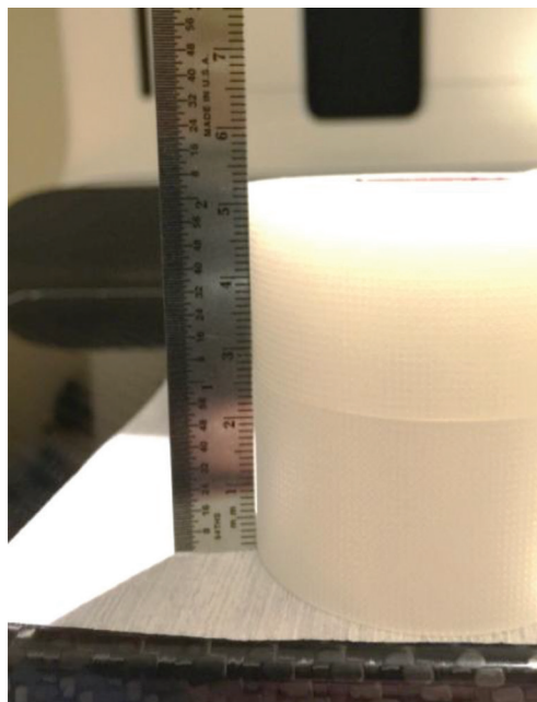
Figure 6. Measuring the width of the compression thickness indicator phantom.
