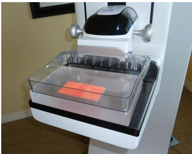
Figure 7. ACR DM Phantom positioned for image acquisition on a 2D system.
