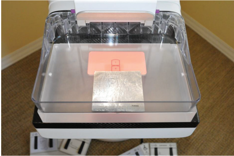
Figure 39. Phantom placed on the image receptor with the aluminum sheet placed correctly.
