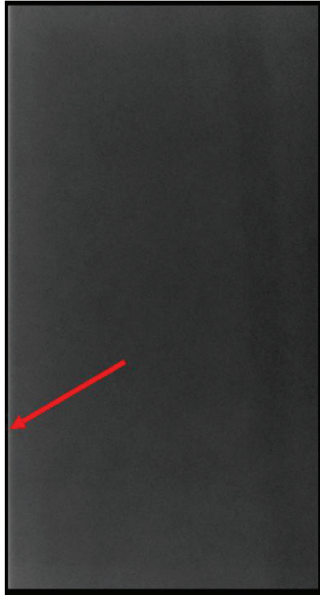
Figure 7. White line along chest-wall edge of image due to collimator misalignment.
