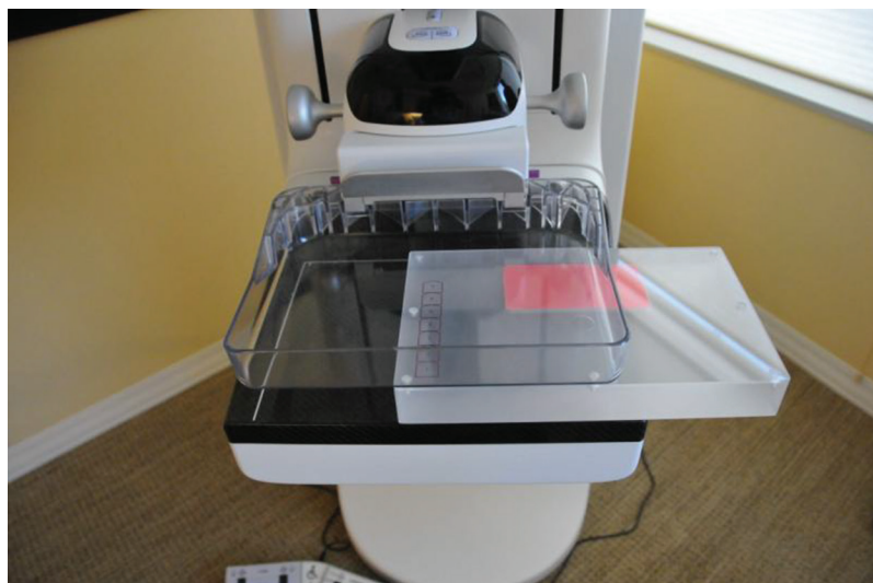
Figure 38. Phantom placed offset on the detector.
