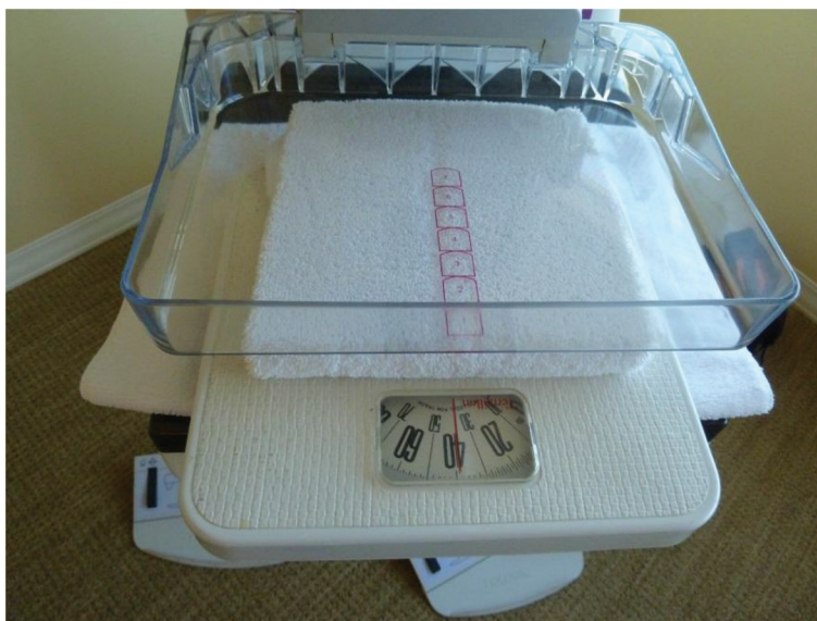
Figure 9. Setup for the compression force test. Note the towel covering the image receptor under the scale and the towel on top of the scale to protect the paddle.
