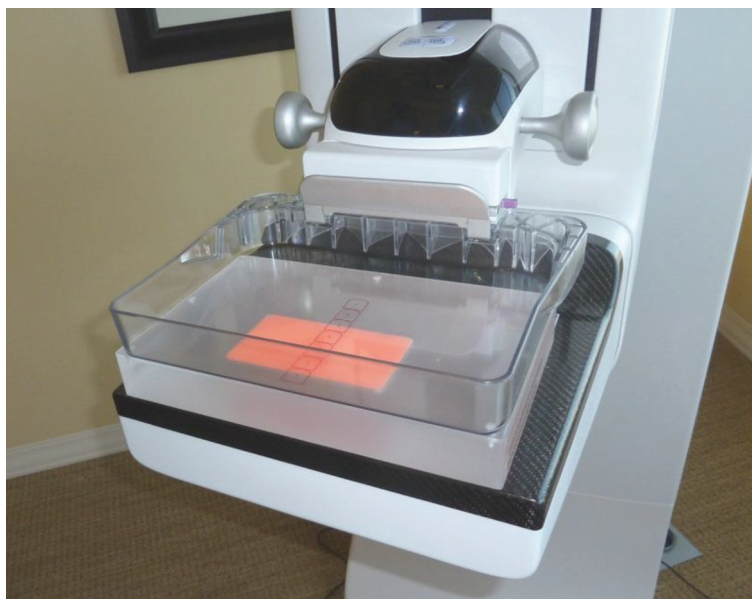
Figure 2. ACR DM Phantom positioned for image acquisition on a 2D system.
