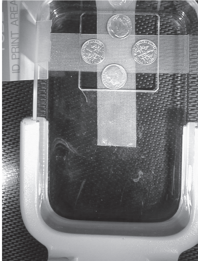
Figure 1. Coins taped to four corners in front of compression plate with edges tangent to edges of biopsy window.
