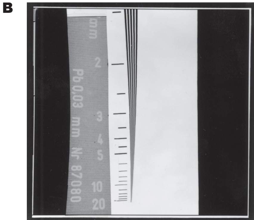
Figures 2A & B. Line Pair patterns photographed from the monitor of a stereotactic breast biopsy system. A: A discrete line pair pattern with a maximum of 10 line pairs per millimeter. B: A continuous line pair pattern with a maximum of 20 line pairs per millimeter.
